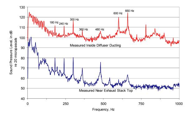
Figure 3: Tonal qualities of advanced turbine designs.
