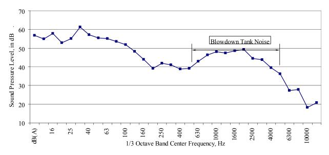
Figure 4: Blowdown tank noise measured within the community without a silencer.
