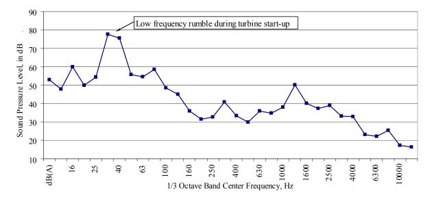
Figure 2: Low frequency rumble of combustion turbine at startup.
